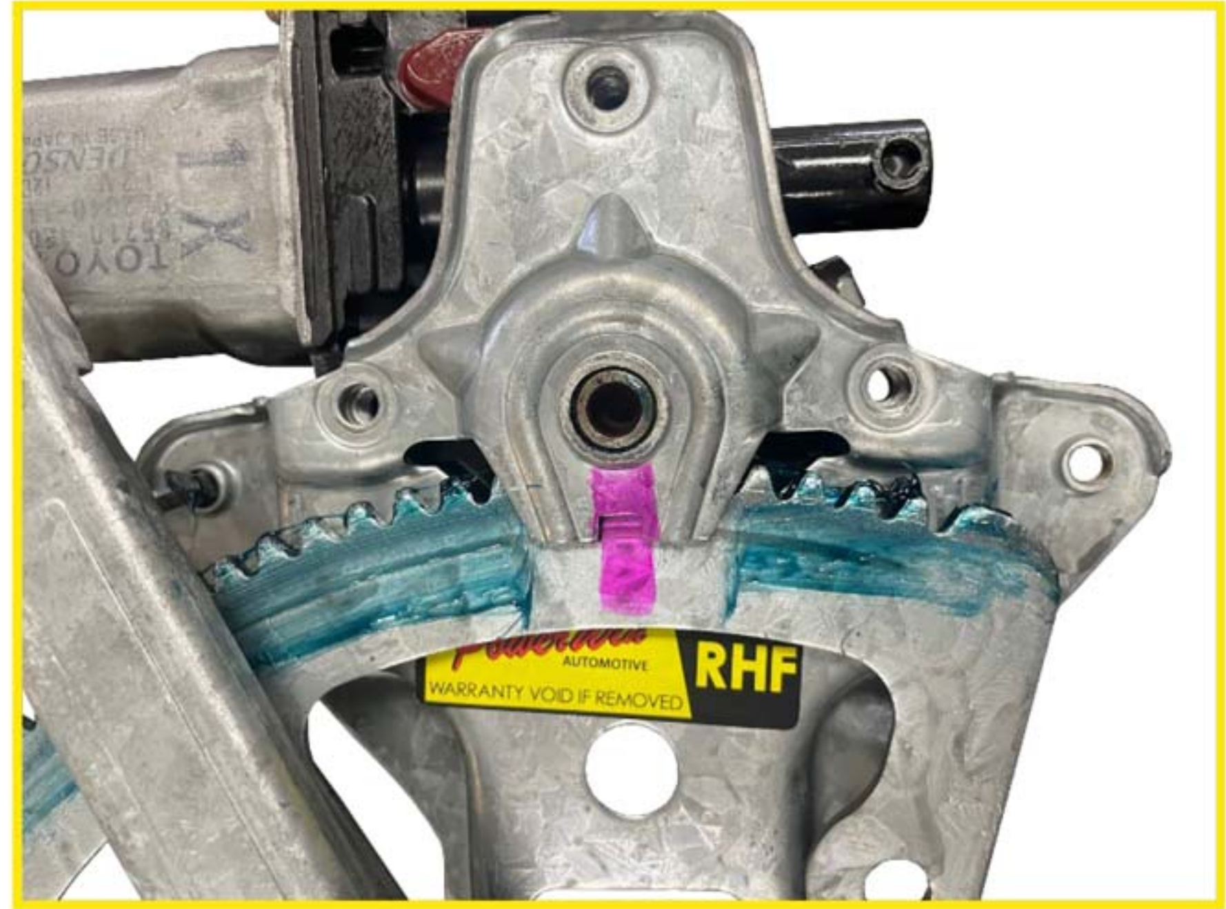
CLEARLY MARK REGULATOR POSITION BEFORE REMOVING MOTOR AS SHOWN IN PICTURE
