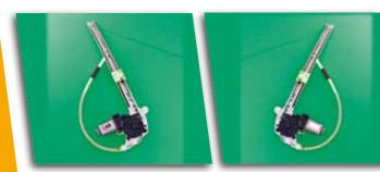
L: WSCELHR **R: WSCERHR Rebuilt Reconditioned** Window Regulator
