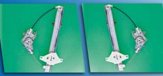
L: WTERRACLHF **R: WTERRACRHF Rebuilt Reconditioned** Window Regulator LHF RHF
