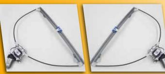
L: WSCELHF R: WSCERHF **Rebuilt Reconditioned** Window Regulator LHF RHF
