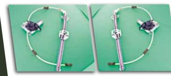
L: WKJLHRCLAMP **R: WKJRHRCLAMP Rebuilt Reconditioned** Window Regulator
