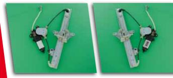
L: WST190LHR R: WST190RHR **Rebuilt Reconditioned** Window Regulator
